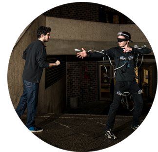
SpiderSense, a wearable tactile vest that alerts the user of obstacles and moving objects
