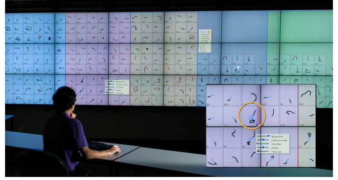
Figure 3. Our trajectory analysis application running on a 19 Megapixels, thin-bezel, tiled 3D display wall. Trajectories are juxtaposed side-by-side and grouped into “bins” depending on their associated meta data. A stereoscopic 3D visual encoding is used to convey spatial and temporal features in the trajectories. The frame at the right bottom of the figure illustrates Coordinated Brushing . A blue paintbrush (circled) is being used to highlight insect movement in the center of the experimental arena.
