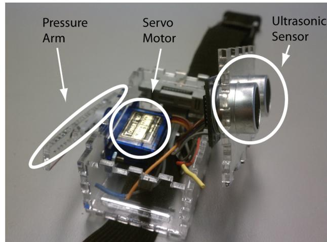
Figure 3: The Sensor Module
