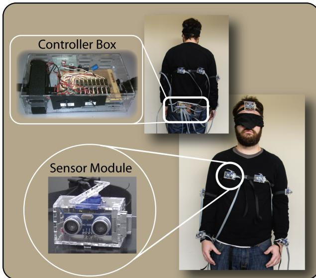
**Figure 2: Positioning of Sensor Modules and Controller Box**
