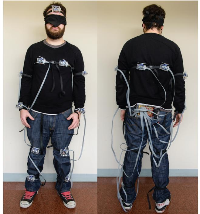
Figure 1: SpiderSense on a blindfolded user
