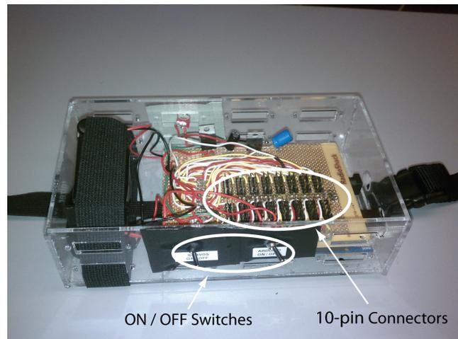
Figure 4: The Controller Box
